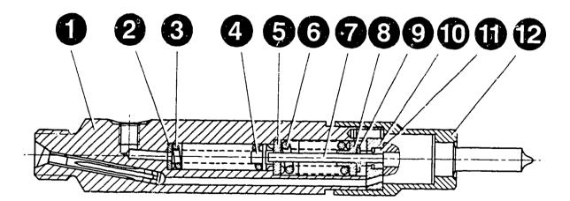
Dual-spring nozzle-holder assembly w i t h needle-motion sensor:
